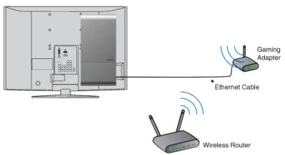
Requirements: Ethernet Cable, Wireless Router, Gaming Adapter or other wireless device serving as a wireless bridge.
